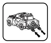
Simultaneously push both exhaust pipes firmly into the body until you hear a click.
